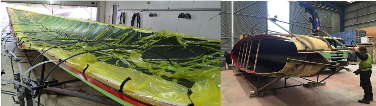
Each hull is constructed of e-glass and foam core using advanced epoxy resin infusion processes. In contrast to these modern methods, traditional aspects will remain clearly visible with each hull lashed together using wooden beams and ropes.
